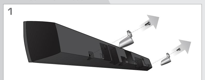
Use a phillips-head screwdriver to remove the screws from the Sound Bar stands. Reinsert the screws for safekeeping. Save the stands for future use.
